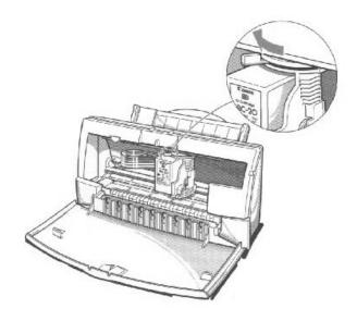
o If you installed the BC-21 Color BJ Cartridge, set the paper thickness lever to the center.
